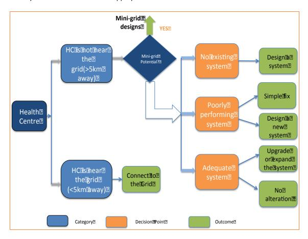
As can be seen, if a system was within 5 km of the grid, a grid connection was recommended<sup>14</sup>. Where there was no system, a poorly performing system or need for system growth, the ASD team designed a new system. Based on the site audits, the team found that with load growth taken into consideration, all sites where grid connection was not viable would require a new solution.
