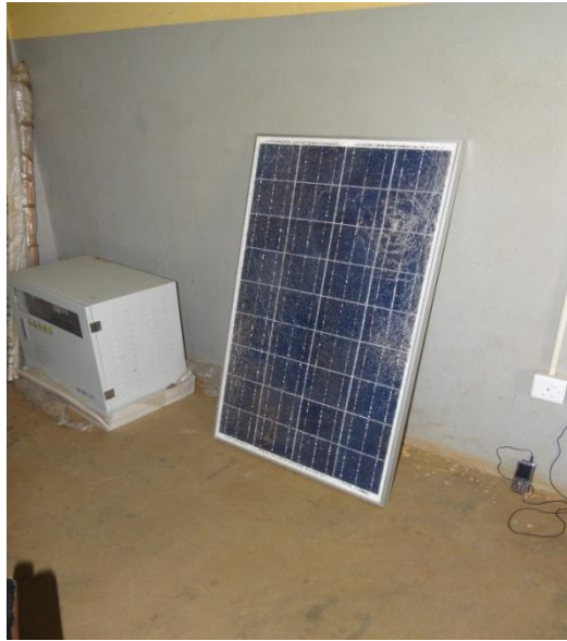
On the left, a visibly cracked Solar panel dumped at Bishop Tarantino College in Lira. On the right, Defective socket at Kithoma Peas S.S.S in Kasese, that cannot accommodate common appliance plugs.
